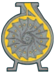
Circular Concentric Casing Internal bypass is drilled through the discharge without breaching the casing wall or creating a potential leak path
